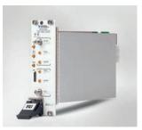
MMPX connectors, operating up to 67 GHz, selected for National Instruments' new generation Vector Signal Transceivers
