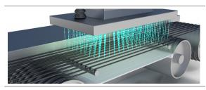
Thanks to e-beam cross-linked insulation, RADOX 125 has 8 times the life of conventional compounds. Even at high temperature, the insulation will not have brittle breakage and thus requires no replacement.
