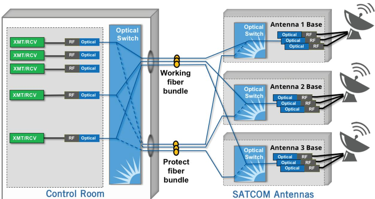
Fig. 1: Typical optically-switched satellite ground station RF-over-Fiber architecture
