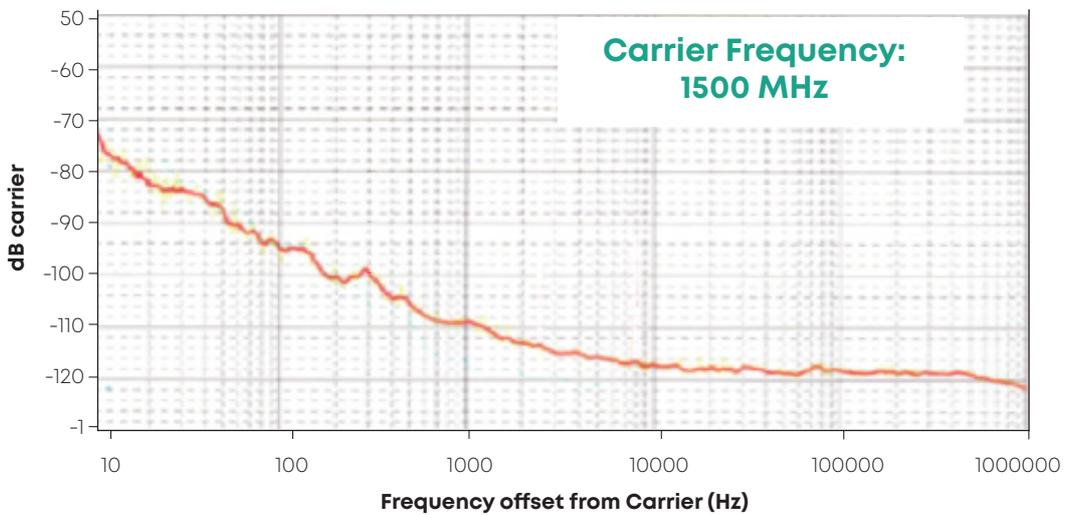
RF link performance with a MEMS switch in the path
