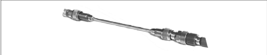
Figure 86 Photograph of DUT No. 2 with N connectors and 50 \Omega termination (left)
