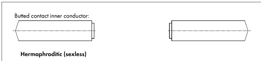
Figure 43 Butted contact inner conductor
