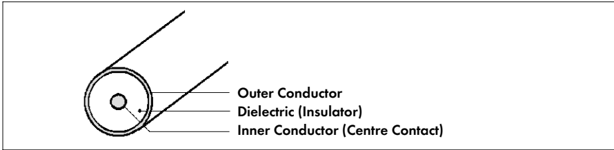
Figure 5 Construction of a RF line
