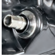
Q-ODC-12 socket on MLUH head
