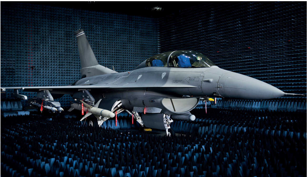
Aircraft on test in anechoic test chamber*
